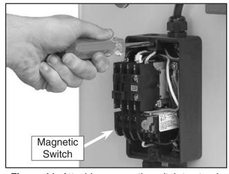
Figure 11. Attaching magnetic switch to stand.
